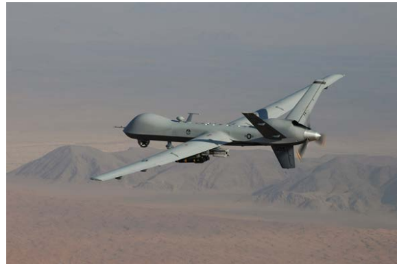
An MQ-9 Reaper, armed with GBU-12 Paveway II laser guided munitions and AGM-114 Hellfire missiles, piloted by Col. Lex Turner flies a combat mission over southern Afghanistan. (U.S. Air Force Photo/Lt. Col. Leslie Pratt)
